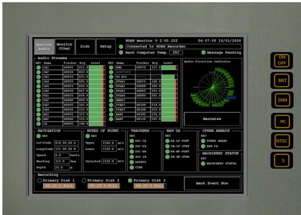
The SDRS is made up of three hardware components; the recording unit, rack computer and flat panel display. The recorder houses the four Hard Disk Drives (HDDs) that are used to continuously capture and record the selected data streams, whilst the flat panel display provides system control and monitoring for the operator.
